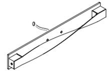
slim backplate OPTIONAL, for direct installation or when using flush mounting kit
