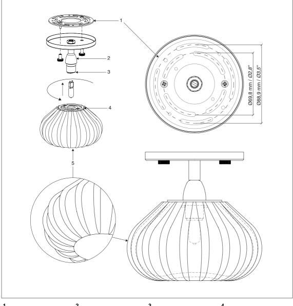
Fixing bracket for iron junction box with their shares of distance between holes.
