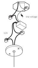
Xenon/LED: Connect the coaxial cable to the open slots in the terminal block on the 12V side of the transformer. Ensure that the braided outer wires are all connected to one 12V output wire and all inner insulated wires are connected to the other or a short will occur.
